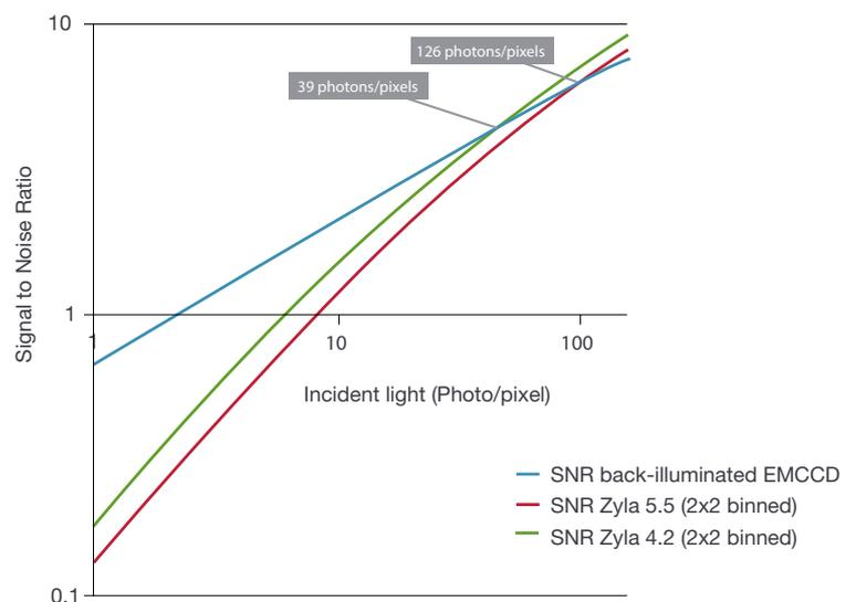
Plot of Signal to Noise Ratio versus Incident Photon Intensity, comparing back-illuminated EMCCD iXon 888 (13 μm pixel size) to 2x2 binned Zyla sCMOS cameras (13 μm pixel size after binning)
